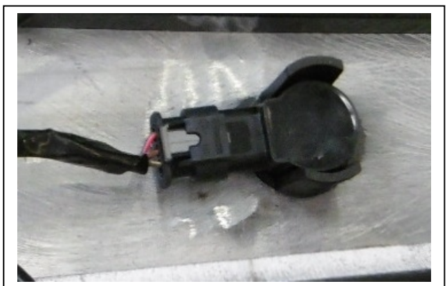
Figure 9: Parking sensor fitted to Protection Bar
