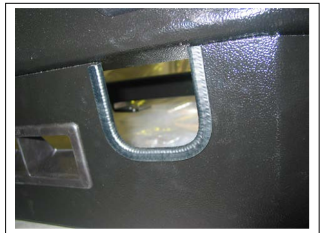
Figure 8: 3mm clip lock trim fitted
