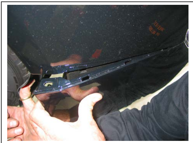
Figure 1: pull bumper rearward and out to release.
